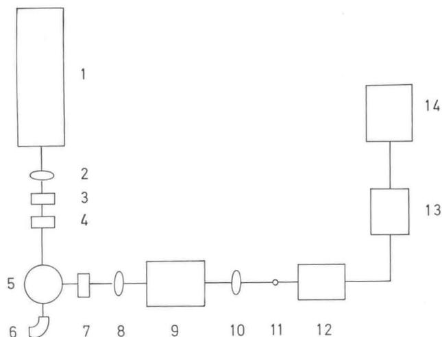
Fig. 1. Light scattering apparatus: (1) argon ion laser; (2) lens A; (3)  $\lambda/2$  plate; (4) Glan-Thompson prism; (5) high pressure optical cell; (6) light trap; (7) polarizer with  $\lambda/4$  plate; (8) lens B; (9) Fabry-Perot interferometer; (10) lens C; (11) pinhole; (12) photomultiplier tube; (13) pulse amplifier and electronic counter; (14) digital recorder.
