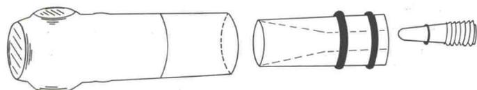
Fig. 2. Liquid sample cell.
